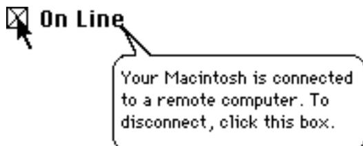
This balloon describes the current state of system, provides an explanation of the option, and describes how to turn off the option.
